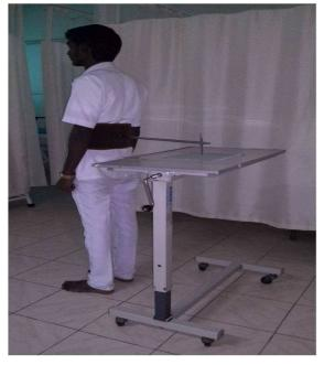
The device (sway meter) consists of inflexible 40 cm long rod with vertically mounted pen at its end. The rod was mounted 20 cm wide metal plate which will be fitted at the level of PSIS (Posterior superior iliac spine) over lower back region of participants by firm belt. Sway meter offers 1 degree of freedom between belt and pen as it's free to move. The pen recorded participants' postural sway on sheet of graph paper which is place over the table.
